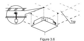
3. Use the hex nuts on the four mounting hooks to adjust and make sure that the unit body is level.
